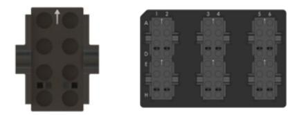
Place the Matrix Tube Strips containing MR01 and MR02 Matrix Reagents into the swing bucket with the 5. barcode side facing right.
