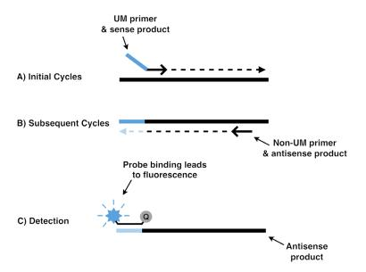
Schematic of the UM chemistry. (A) During initial cycles of PCR, the UM primer with UM adapter (in blue) binds to the template and extends. (B) In subsequent PCR cycles, the non-UM primer binds to the sense template (now with UM adapter) and extends to create an UM probe complementary sequence. (C) The detection of target amplicon occurs via hybridization of the UM probe to target amplicon.
