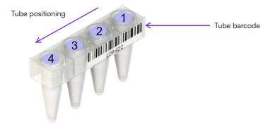
2. Dispense **40** µL of **MR01 Matrix Reagent** (PR0001) into the bottom of each Matrix Tube Strip. Pipette to the first stop to prevent bubble formation.
