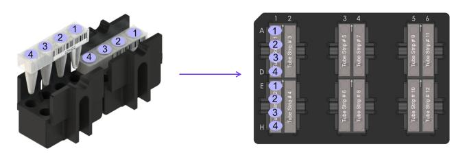
Place Matrix Column Strips (Cat # KTOOO1A) into Matrix Tube Strips with the black orientation dot facing right . 6.
